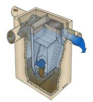
The Terre Kleen™ separator is contained within a HS-25 precast concrete structure. Each stacked overlapping plate is inclined 55°, creating a settling cell containing 6.4 ft² of horizontally projected sedimentation surface area.
