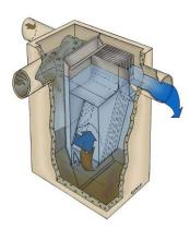
The Terre Kleen<sup>TM</sup> separator is contained within a HS-25 precast concrete structure. Each stacked overlapping plate is inclined 55°, creating a settling cell containing 6.4  $ft^2$  of horizontally projected sedimentation surface area.
